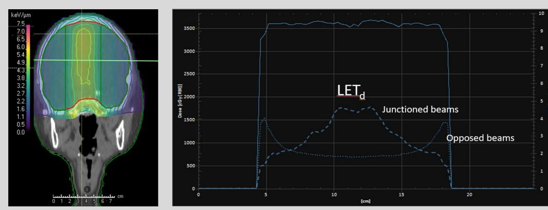
LET<sub>d</sub> for junctioned fieldsComparison of LET<sub>d</sub> across whole brain for standard parallel opposed fields and lateral junctioned fields.
